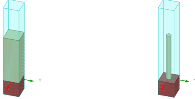
Figure 4.14 HFSS model: (left) vegetation canopy having effective permittivity (right) vegetation canopy consisting of infinite number of finite-length cylinders.
